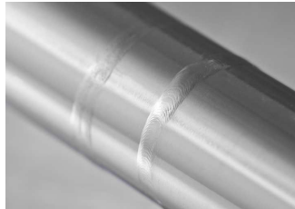
Tubesystem welded material 1.4435 Untreated and after chemical pickling
