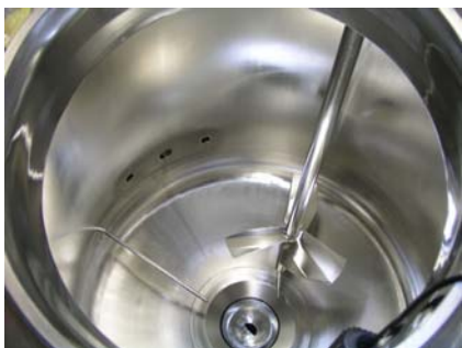
Stainless steel tank, material 1.4435 before and after surface treatment on-site with optimized Henkel-procedure
